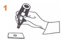
Engage all threads of the Rivnut Fastener on the pull up stud. Advance anvil until it is tight on head of Rivnut. Insert Rivnut in hole.
